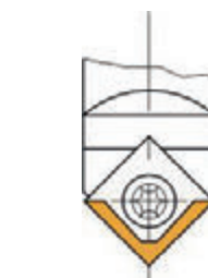
Available area for profiling (1:1) Surface à profiler (1:1)
