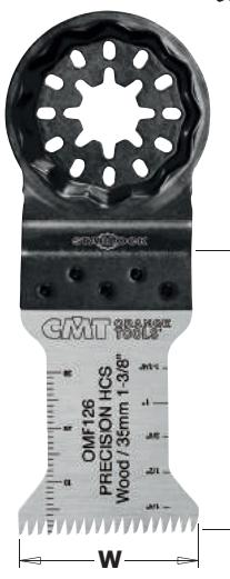
**35mm Precision Cut, Japanese toothing for Wood****FEATURES:** HCS with "Japanese" double-row pattern, hardened teeth**MATERIAL:** wood up to 50mm, plasterboard and soft plastics.**APPLICATION:** plunge easily at any point in the material.
