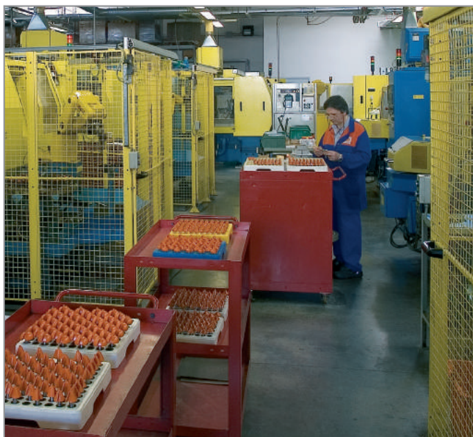
Loading the automated multi-axis CNC sharpening machines.
