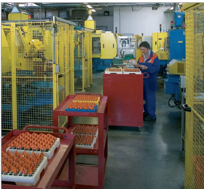
Loading the automated multi-axis CNC sharpening machines.
